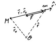
Figure 2.1: Vector diagram showing the geometry of the gravitational attraction.
