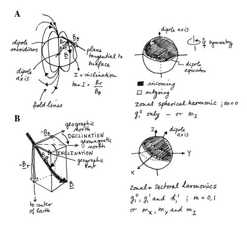
Figure 3.5: Geographic and geomagnetic reference frames and how to represent the dipole with spherical harmonics coefficients in both references systems.
