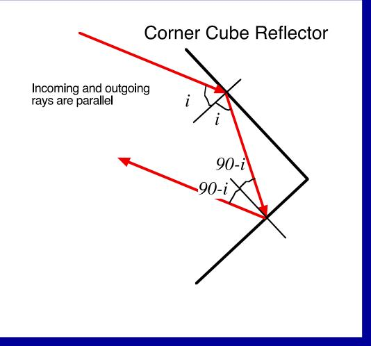
The return angle is twice the corner angle For 90 degree corner, return is 180 degrees.
