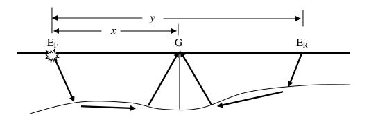
Derive reliable  $v_2$  when the interface varies:
