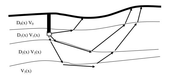
**Objective**: given traveltimes observed at the surface, invert layer depths  $D_i(x)$ , and velocity  $V_i(x)$
