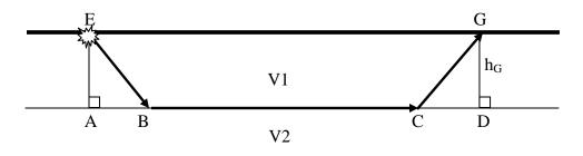
Total delay time for source and receiver:  $T_{EG} = T_E + T_G$  (1)
