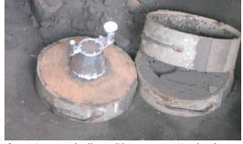
A cast corn sheller with sprues attached.
