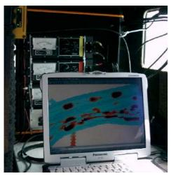
The system records the data directly into a commercial laptop at 20 times per second, which allows a faster recording over conventional data-logging systems and less chance of human error. The data is stored directly into an Access database file for projection into standard GIS systems.
