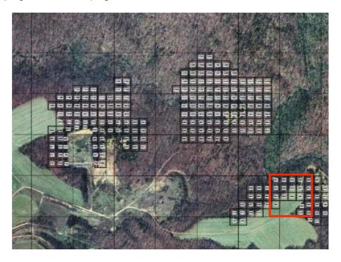
The Overview can be broken down into larger grids, which would be highlighted when the REST filters indicate a presence of explosives. The individual 50x50 or 100x100 sub-grids can then be identified through the higher resolution settings. Anything obviously noticeable would also be entered on the map, so a living system is developed
