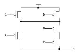
B. Assuming the correct pullup circuitry is added to the diagram above, give a minimal sum-of-products expression for F(A,B,C,D).
