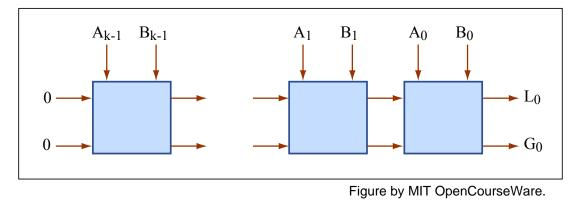
The most significant bits are supplied as Ak-1 and Bk-1, and the least significant bits are A0 and B0.
