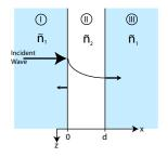
Figure 2: 1D schematic of coupling via evanescent field.
