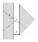
Figure 1: Schematic of frustrated internal reflection.
