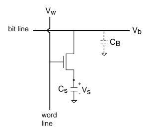
In this DRAM cell, the information is stored in the form of charge in the capacitor  $C_s$ . If the voltage across the capacitor  $V_s$  is HI, then a "1" is stored. If  $V_s$  is LO, a "0" is stored.
