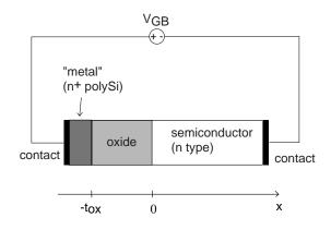
The doping level in the substrate (or body) is  $N_D = 10^{17} \ cm^{-3}$ . The doping level in the gate is  $N_D^+ = 10^{20} \ cm^{-3}$ .
