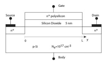
A capacitance voltage curve of the  $n^+$  poly-silicon gate MOSFET was taken by connecting the source, drain and body terminals together. A voltage was applied between the gate and the body.
