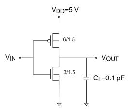
In the above diagram, the two numbers next to each transistor give its gate dimensions (width/length) in microns. In solving this problem, assume that  $C_L$  is the dominant capacitance in this circuit. All other capacitances can be neglected next to  $C_L$ .
