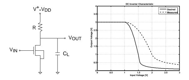
The circuit parameters under suspicion are the MOSFET gate width to length ratio, W/L, the MOSFET gate oxide thickness,  $t_{ox}$ , the MOSFET body doping level,  $N_a$ , and the pull-up resistance, R. Further, assume that one and only one of these four parameters was incorrectly fabricated.
