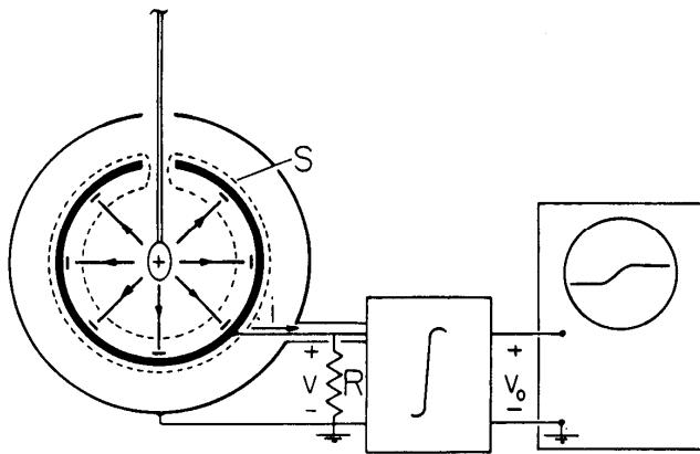
**Figure 1.5.5** When a charge  $q$  is introduced into an essentially grounded metal sphere, a charge  $-q$  is induced on its inner surface. The integral form of charge conservation, applied to the surface  $S$ , shows that  $i = dq/dt$ . The net excursion of the integrated signal is then a direct measurement of  $q$ .
