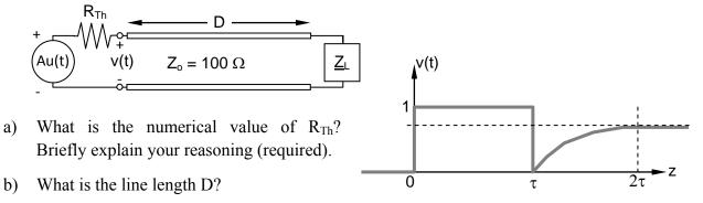
c) Diagram a simple load at the end of the line that could produce this response; it is not necessary to compute element values. Simply label your components as R, L, or C, as necessary.
