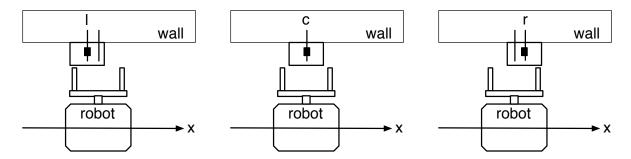
Note that these represent positions of the **center of the block relative to the center of the gripper**.
