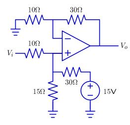
Let  $V_+$  and  $V_-$  represent the voltages at the positive and negative input terminals of the op amp. Determine an expression for  $V_-$  in terms of  $V_o$ .
