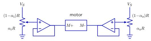
The dependence of the pot resistances on shaft angle is given in terms of  $\alpha$ , which varies from 0 (most counterclockwise position) to 1 (most clockwise position). The resistance of the lower part of the pot is  $\alpha R$  and that of the upper part is  $(1 - \alpha)R$ , where  $R = 1000\Omega$ .
