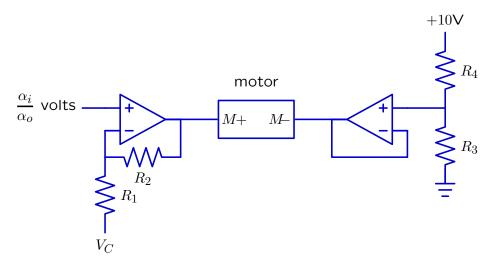
so that the motorshaft angle (which is proportional to  $\alpha_o$ ) will track the input pot angle (which is proportional to  $\alpha_i$ ).
