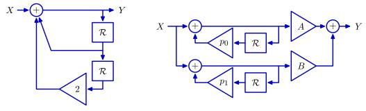
It is possible to choose coefficients for the block diagram on the right so that the systems represented by the left and right block diagrams are "equivalent".<sup>1</sup>
