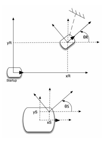
It is useful when computing this to think about first finding the location of the hit point relative to the robot and then computing the position of that point relative to the global odometry frame.
