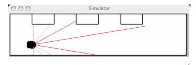
Part of the robot model is an error model for the sonar readings. Our error model for sonar readings will have a similar structure to the error model for observing colors in the hallway: we determine the sonar observation we would expect to see in each state, if our observations were perfect, and then use that as the basis for constructing a distribution over possible observations.
