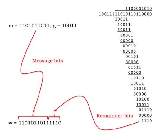
Figure 6-3: CRC computations using "long division".
