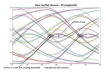
Figure 11-10: Eye diagrams for a channel with a slow rise/fall for 33 (top) and 20 (bottom) samples per bit. Notice how the eye is wider when the number of samples per bit is large, because each step response has time to settle before the response to the next step appears.
