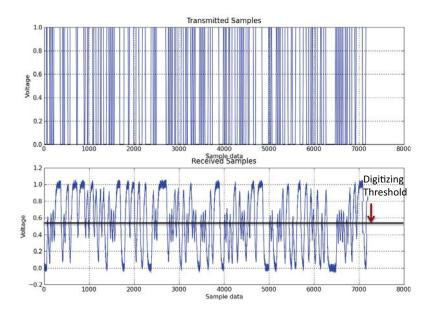
Figure 11-11: Received signals in the presence of ISI. Is the number of samples per bit "just right"? And what threshold should be used to determine the transmitted bit? It's hard to answer these question from this picture. An eye diagram sheds better light.
