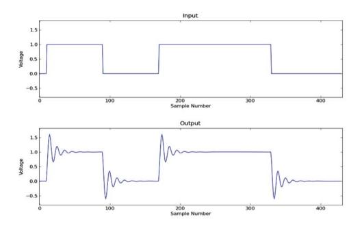
Figure 11-2: A channel showing "ringing".
