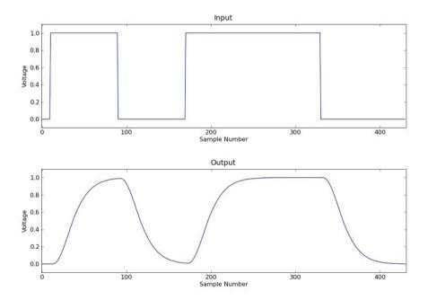
Figure 11-1: On-off signaling at the channel input produces a channel output that takes a non-zero time to rise or fall, and to settle at 1 or 0.
