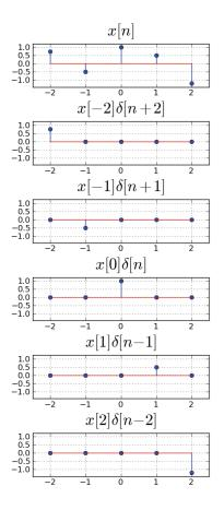
Figure 11-5: A discrete-time signal can be decomposed into a sum of time-shifted, scaled unit-sample functions:  $x[n] = \sum_{k=-\infty}^{\infty} x[k]\delta[n-k]$ .
