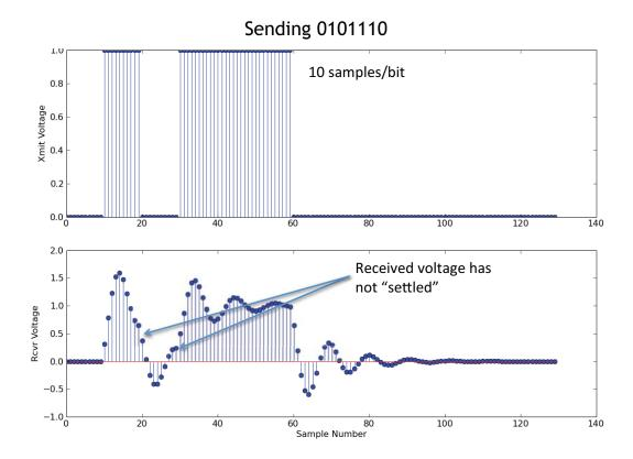
Figure 11-3: The effects of rise/fall time and ringing on the received signal.
