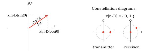
Figure 14-12: Quadrature demodulation. The term "constellation diagram" refers to the values that the sender can send, in this case just 0 and 1 volts. The receiver's steps are shown in the picture.
