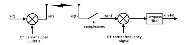
We use the symbols y[n] and x[n] to denote the discrete-time (DT) signals that would have been obtained by respectively sampling y(t) and x(t) in Equation (14.9) at  $f_s$ samples/sec; more specifically, the signals are sampled at the discrete time instants  $t = n(1/f_s)$ . Thus
