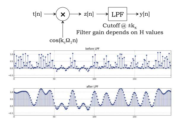
Figure 14-9: Demodulation steps: the no-delay case (top). LPF is a lowpass filter. The graphs show the time-domain representations before and after the LPF.
