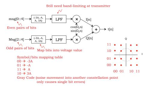
Figure 14-16: Quadrature Amplitude Modulation (QAM).
