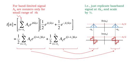
Figure 14-5: Illustrating the heterodyne principle.
