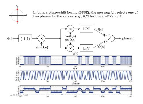
Figure 14-14: Binary Phase Shift Keying (BPSK).
