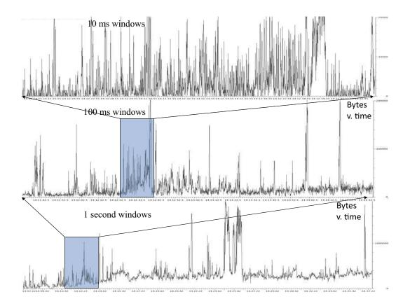
Figure 16-9: Traffic bursts at different time-scales, showing some smoothing. Bursts still persist, though.
