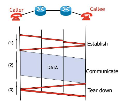
Figure 16-4: Circuit switching requires setup and teardown phases.
