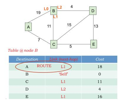
Figure 17-2: A simple network topology showing the routing table at node B. The route for a destination is marked with an oval. The three links at node B are L0, L1, and L2; these names aren't visible at the other nodes but are internal to node B.
