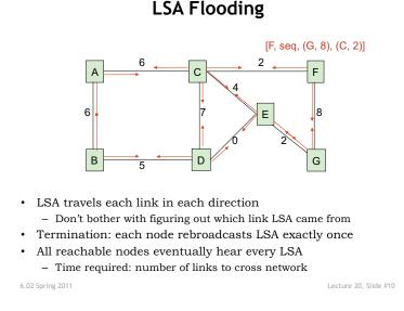
Figure 17-5: Link-state advertisement from node F in a network. The arrows show the same advertisement being re-broadcast (at different points in time) as part of the flooding process once per node, along all of the links connected to the node. The link state is shown in this example for one node; in practice, there is one of these originating from each node in the network, and re-broadcast by the other nodes.
