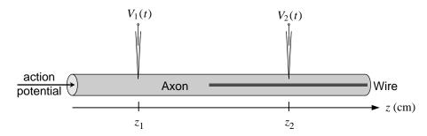
The wire is so thin that its volume can be ignored. The axon (500  $\mu$ m diameter) is electrically stimulated to produce a propagated action potential traveling in the +z direction. The action potential is recorded at two intracellular sites:  $V_1(t)$  is recorded at  $z = z_1$  and  $V_2(t)$  is recorded at  $z = z_2$ . The distance between the stimulus electrode (not shown) and  $z_1$  is 2 cm. Results are shown in the following figure.
