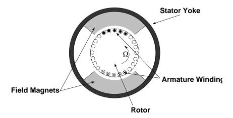
Figure 17: PM Commutator Machine
