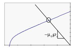
Figure 15: Load Line, Unit Permeance Analysis
