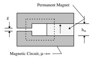
Figure 14: Permanent Magnet Driving an Air-Gap
