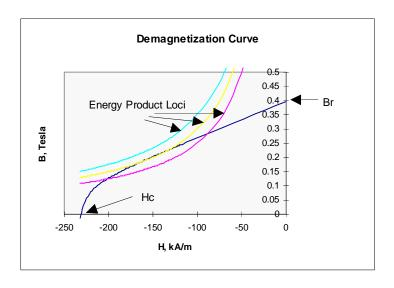
Figure 12: Demagnetization Curve
