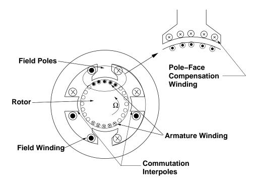
Figure 10: Pole Face Compensation Winding
