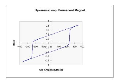
Figure 11: Hysteresis Loop Of Ceramic Permanent Magnet
