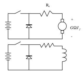
Figure 5: Two-Chopper, separately excited machine hookup
