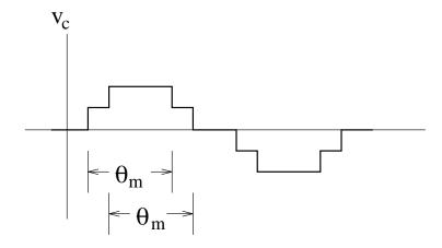
Figure 19: Voltage Induced in a Coil
