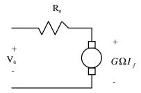
Figure 3: DC Machine Equivalent Circuit
