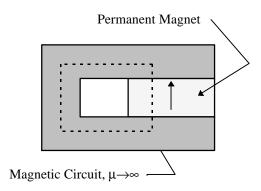
Figure 13: Permanent Magnet in Magnetic Circuit
