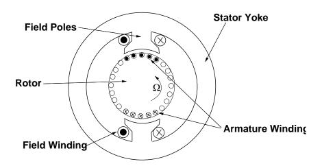
Figure 1: Wound-Field DC Machine Geometry
