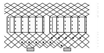
Figure 7: Commutator and Current Paths
