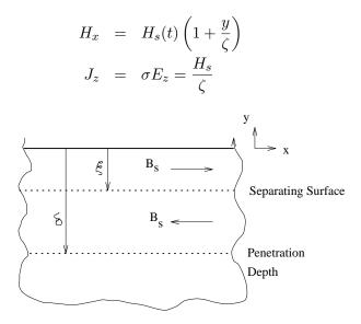
Figure 13: Separating Surface and Penetration Depth
