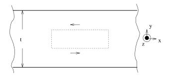
Figure 11: Lamination Section for Loss Calculation
