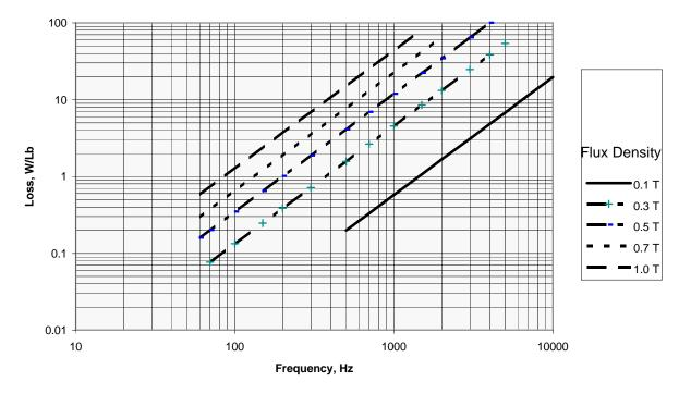
Figure 15: Steel Sheet Core Loss Fit vs. Flux Density and Frequency
