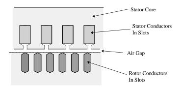
Figure 4: Windings in Slots
