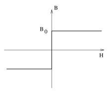
Figure 12: Idealized Saturating Characteristic
