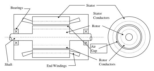
Figure 3: Form of Electric Machine
