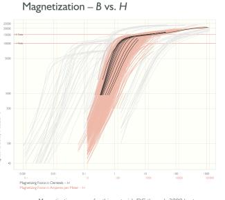
Magnetization curves for this material, DC through 2000 hertz All non-oriented silicon steels All other materials Total core loss curves for this material, 50 through 2000 hertz All non-oriented silicon steels All other materials
