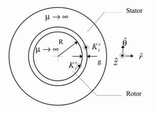
Figure 1: Elementary Machine Model: Axial View
