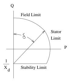
Figure 6: Synchronous Generator Capability Diagram
