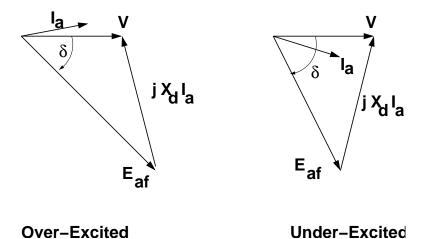
Figure 3: Motor Operation, Under- and Over- Excited
