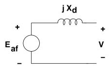
Figure 2: Round Rotor Synchronous Machine Equivalent Circuit
