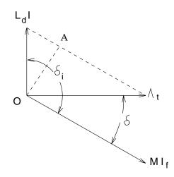
Figure 5: Synchronous Machine Phasor Addition
