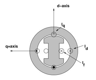
Figure 8: Cartoon of a Salient Pole Synchronous Machine
