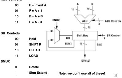
We could control this with one large FSM, but it seems reasonable to break the control down to several smaller (more easily developed and tested) FSM's, which must then be coordinated
