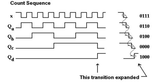
The effect of each input transition must affect all bits, and it does this by rippling through from LSB to MSB
