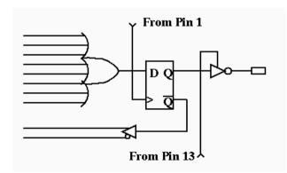
Note that in this case the 'feedback' is from the register, not the pin. Pin 1 is now dedicated to being the clock input and is not available as a regular input.
