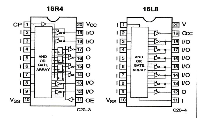
Here is a schematic diagram for the 16L8: we can learn more about this by considering its parts.
