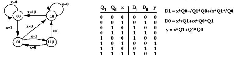
It is straightforward to build a truth table for 'next state' based on 'present state' and input. The output is also derived from the same variables.
