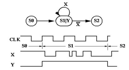
Clock speed is limited by FF delay, Combinatoric delay and setup time. New state is determined by inputs and old state just BEFORE clock edge
