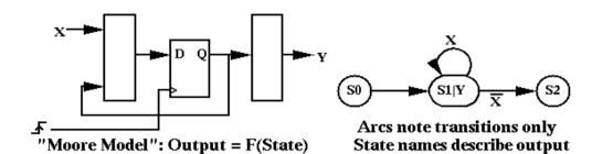
On the other hand, if the input is used ONLY in the next-state logic, the output is fixed during each clock cycle and only changes after the clock edge.
