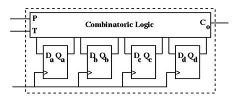
Synchronous Counters: reduce ripple by setting all bits at once
