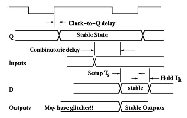
We have automated procedures to build the logic foe finite state machines, but here is an example of a very simple machine.
