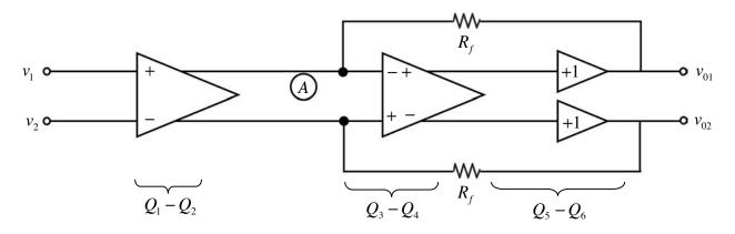
If we look in the course reader, we'll see that the gain of the amplifier formed by  $Q_3 - Q_4$  is on the order of 100. The data sheet specs the output swing at  $V_{p-p}$ . What this means is that the differential voltage swing at point (A) is only  $47mV_{p-p}$ ...it is a low-swing node!
