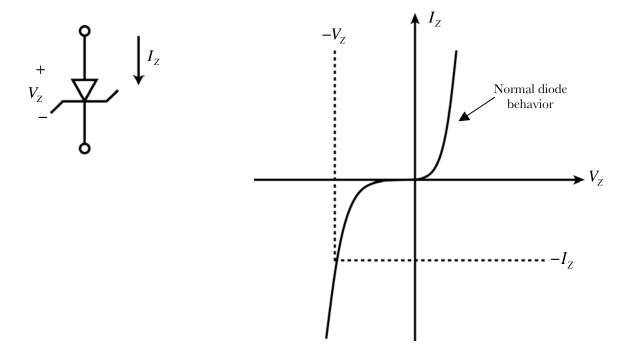
By choosing the doping profile of the pn junction, the actual breakdown mechanism traces to one of two phenomena:
