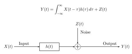
Figure 1.5: Linear Gaussian channel model.
