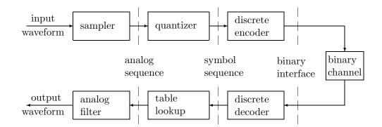
Figure 1.3: Breaking the source coding/decoding layer into 3 layers for a waveform source. The input side of the outermost layer converts the waveform into a sequence of samples and output side converts the recovered samples back to the waveform. The quantizer then converts each sample into one of a finite set of symbols, and the peer module recreates the sample (with some distortion). Finally the inner layer encodes the sequence of symbols into binary digits.
