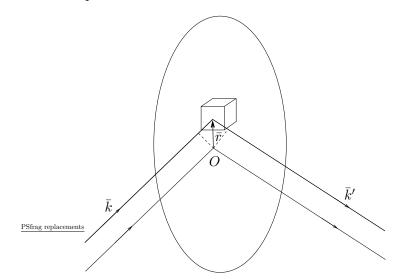
**Figure 5:** Diffraction from an elementary volume of a periodic medium:  $\bar{k}$  is the wavevector of the incident wave whereas  $\bar{k}'$  is the wavevector of the diffracted wave.
