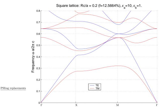
Figure 8: Dispersion diagram for the photonic crystal of Fig. 7.
