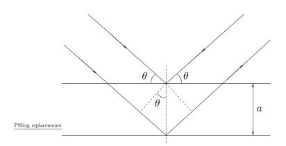
Figure 4: Schematic representation of Bragg diffraction. Maximal diffraction occurs at  $2a\sin\theta = n\lambda$  where  $\lambda$  is the wavelength of the electromagnetic wave and n is an integer.
