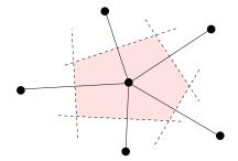
**Figure 1:** Wigner-Seitz cell for an arbitrary position of points: the cell is constructed by joining the center element to its closest neighbors and drawing perpendicular lines from to the center of these segments. The polygon thus created is the smallest repeatable cell of the periodic lattice, and is defined as the Wigner-Seitz cell.
