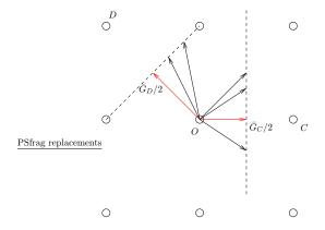
Figure 6: Graphical representation of Eq. (17): each vector  $\bar{k}$  (black vector) with its tip on a dashed line (not all represented) will satisfy the equation. Graphically: all those  $\bar{k}$  have the same projection on the generating vector  $\bar{G}/2$  (red vector).
