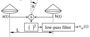
b) Assume we must use a diode with  $i = v^2 + cv^3$  instead of the illustrated square-law device, and that a(t) and b(t) are narrowband signals centered at 100 MHz. How might you change the circuit (minimally, if at all) so that the interferometer still works? Note that the same issue arises in communications receivers employing matched filters.
