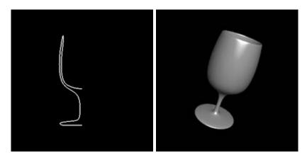
The images below show an example of a generalized cylinder. On the left is what we'll call the *sweep* curve, and the surface is defined by sweeping a *profile* curve along the sweep curve. Here, the profile curve is chosen to be a circle, but your implementation should also support arbitrary two-dimensional curves.
