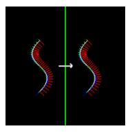
Here, the normals that were once facing towards the *y*-axis are now facing away! Rather than try to handle both cases, we will assume for this assignment that the profile curve is always on the *left* of the *y*-axis (that is, all points on the curve will have a negative *x*-coordinate).
