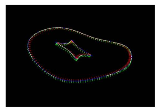
The small curve is chosen to be the profile curve, and the large one is chosen to be the sweep curve. The resulting generalized cylinder is shown below.
