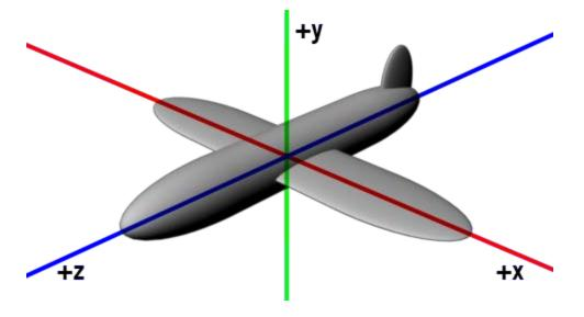
And let's say that we wanted to align the z-axis of the airplane with the tangent  $\mathbf{T}$ , the x-axis with the normal  $\mathbf{N}$ , the y-direction with the binormal  $\mathbf{B}$ , and have the plane at position  $\mathbf{V}$ . This can be achieved with the following transformation matrix:
