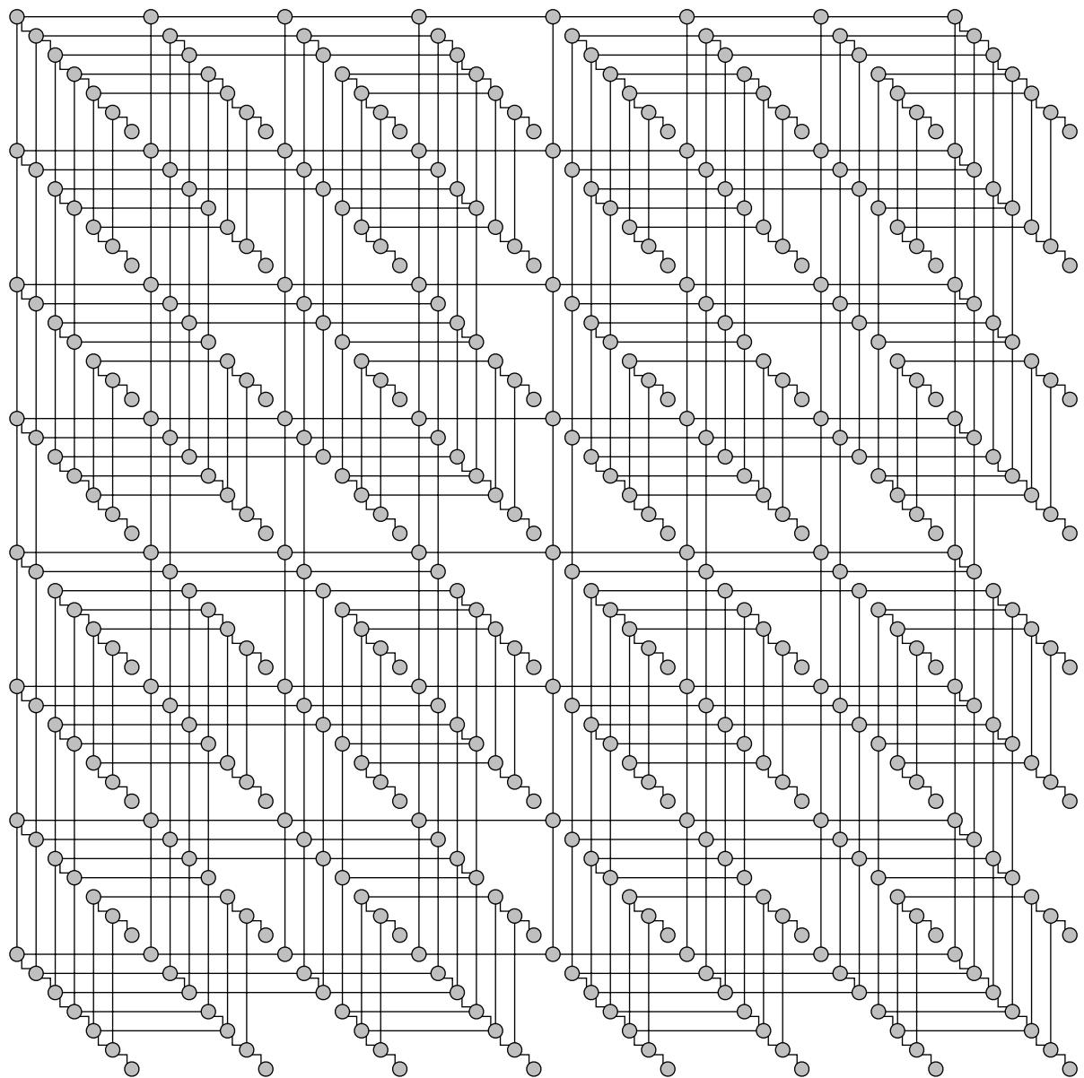
Wires should be rectilinear on a grid, and your layouts should have asymptotically optimal area.
