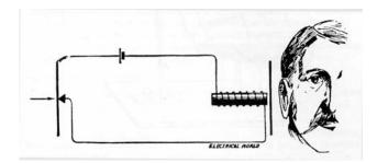
Fig. 4.3: Bourseul's make-and-break concept. (This image is public domain and is not protected by copyright.)
