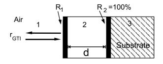
Using  $r_1 = -\sqrt{R_1}$ ,  $r_2 = -\sqrt{R_2} = -1$  and assuming that medium 2 has a refractive index 1, the following expression for the amplitude reflectivity can be found:
