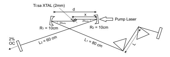
Gain Medium: The Ti:sapphire crystal will be used for the gain medium. The gain bandwidth of Ti:sapphire is  $\Omega_g = 2\pi \times 43$  THz with a center wavelength of 800 nm. The crystal length is t = 2 mm. The refractive index of the crystal is 1.76 at 800 nm. For a rough estimation of the pulsed operation, assume the fast saturable absorber coefficient  $\gamma$  and the self-phase modulation coefficient  $\delta$  are:  $\gamma = 10^{-7}/W$  and  $\delta = 10^{-6}/W$ .
