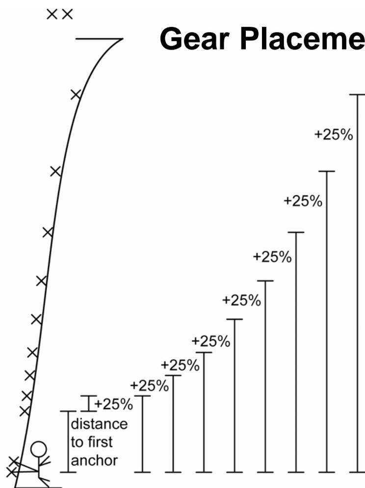
Anchor placement for trad leading based on the analysis by Stephen Attaway. To prevent gear failure, the leader must place gear when 25% above the last gear. This analysis does not include margin for the possible failure of the top gear, by poor placement or misadventure. In this example, if the first gear is 2 meters above the anchor, the total pitch length is less than 20 meters.
