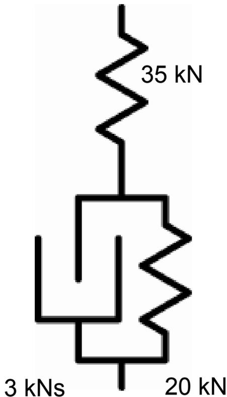
Spring in series with spring/dashpot parallel combo
