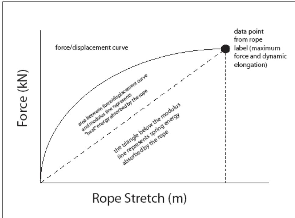
The hang tag provides the force and % rope extension. The length of rope and the fall height are defined by the test standard.
