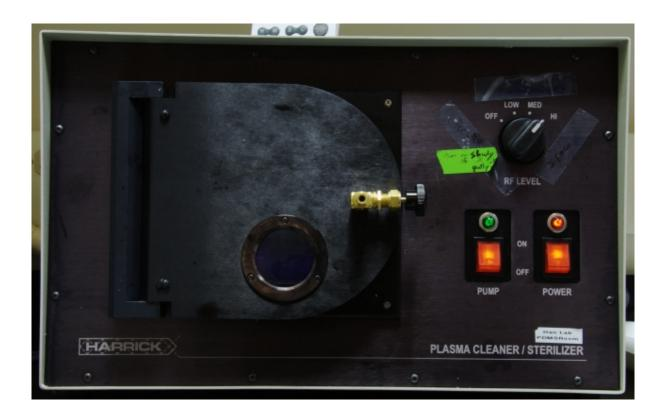
The vacuum pump has two indicators that tell you when the vacuum is ready. First, a light on the pump itself turns from yellow to green. Second, the vacuum gauge shows that the pressure drops to about 65 mbar (i.e., 65/1000 of atmospheric pressure) and stabilizes there. At this point you can turn the RF signal on to the highest setting. When you do so, you should see a purple glow coming from the inside of the chamber.
