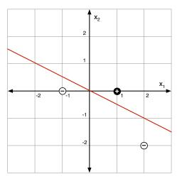
Data points are: Negative: (-1, 0) (2, -2) Positive: (1, 0). Assume that the points are examined in the order given here. Recall that the perceptron algorithm uses the extended form of the data points in which a 1 is added as the 0th component.
