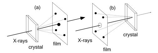
Figure 9 Laue diffraction in (a) transmission and (b) back-reflection mode
