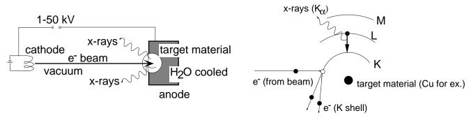
Figure 2 Generation of x-rays
