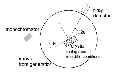
sample (ground to a powder) into the center of a rotating stage and expose it to a monochromatic X-ray beam. The sample is rotated into diffraction condition and the diffraction angle determined. In the Debye-Scherrer method (fig.12) the sample
