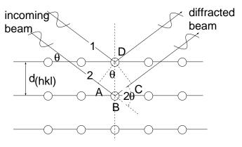
Figure 8 Bragg's law, assuming the planes of atoms behave as reflecting planes.
