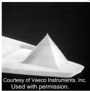
Figure 2 An SEM micrograph of a typical AFM cantilever. (Veeco Instruments,
