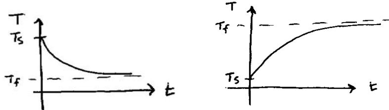
Transient Heat Conduction: depends on position and time
