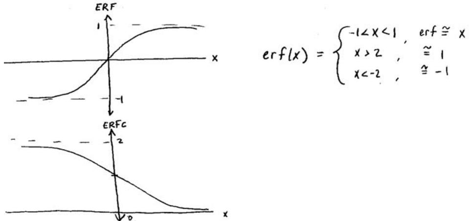
$$T(x) = (T_1 - T_0) \text{erfc} \left( \frac{x}{2\sqrt{\alpha t}} \right) + T_0$$
