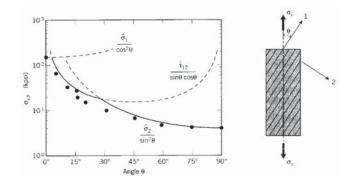
Figure 3: Stress applied at an angle to the fibers in a one-dimensional ply.
