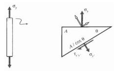
Figure 2: An inclined plane in a tensile specimen.
