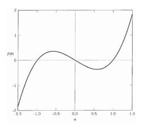
Figure 12: The characteristic equation for  $\tau_{xy} = 1$ , all other stresses zero.
