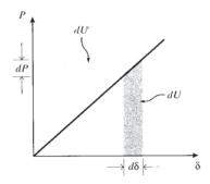
Figure 9: Increments of strain and complimentary strain energy.
