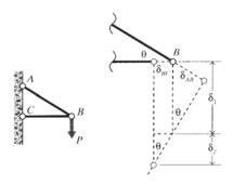
Figure 8: Displacements in the two-element truss.
