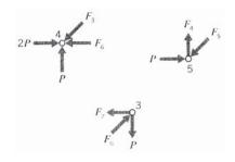
Figure 6: Individual joint diagrams.
