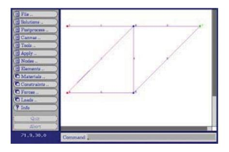
Figure 16: The six-element truss.
