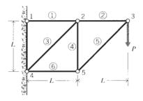
Figure 4: A six-element truss.
