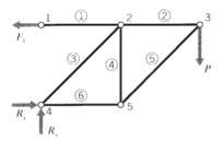
Figure 5: Free-body diagram of six-element truss
