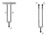
Figure 10: Two truss elements in parallel.
