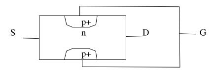
For  $V_G = 0$  it is a linear resistor. However, applying  $V_{SD}$  causes pinch-off (i.e. the depletion regions touch) and no more current  $I_{SD}$  can flow. Applying a negative  $V_G$  makes pinchoff occur earlier. Beyond pinchoff, a small change in  $V_G$  causes a large change in  $V_{SD}$ .
