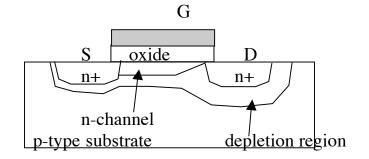
Source and substrate are grounded. Applying a large positive  $V_G$  creates an n-channel which conducts current between S and D.
