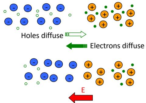
An electric field forms due to the deviation from charge neutrality
