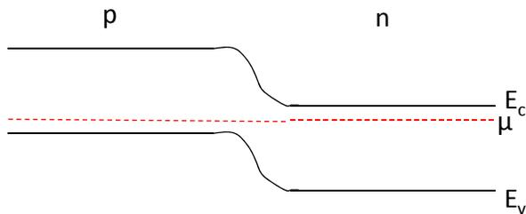
Carriers flow under driving force of diffusion until  $\mu$  is horizontal
