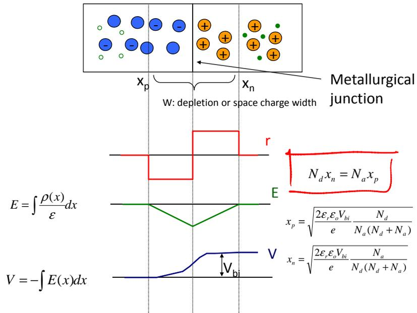
What is the built-in voltage  $V_{bi}$ ?
