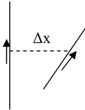
Case B: Two edge dislocations separated by a distance  $\Delta x$ , at  $90^\circ$  from one another. (The picture is drawn in perspective; the dislocations are parallel to the y and z axes)
