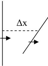
Case C: An edge and a screw dislocation separated by a distance  $\Delta x$ , at  $90^\circ$  from one another. (The picture is drawn in perspective; the dislocations are parallel to the y and z axes)
