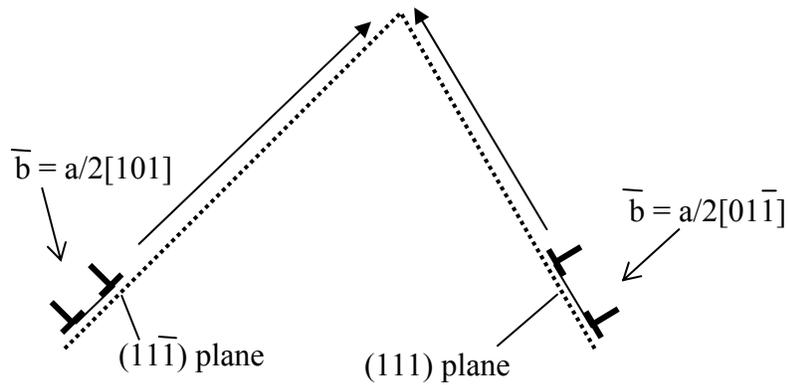
The two initial dislocations have Burgers vectors of  $a/2\langle 110 \rangle$  type as shown; however, as the picture implies, these dislocations are actually separated into partials of  $a/6\langle 211 \rangle$  type.
